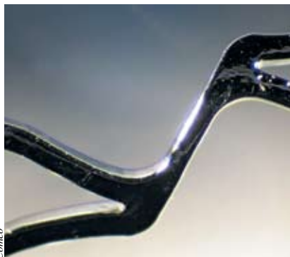
These images show a magnified section of a nitinol stent before microabrasive blasting (top), after blasting (middle) and, finally, after electropolishing.
