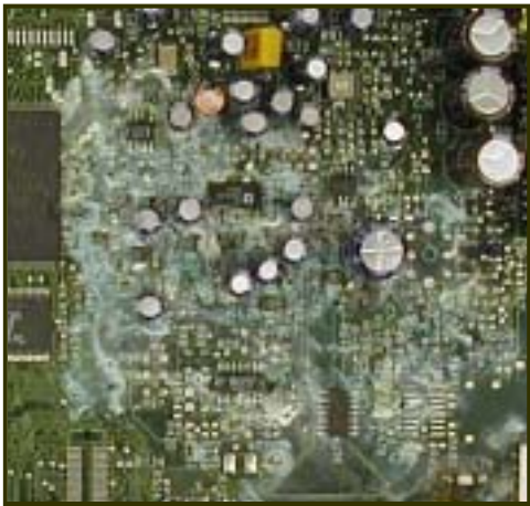
PC board prior to cleaning with the MicroBlaster
