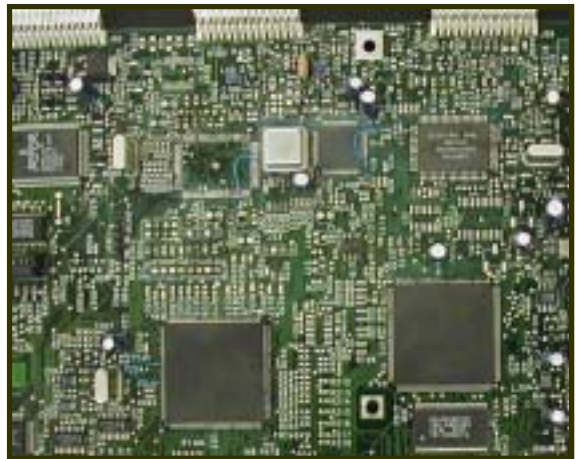
PC board after micro-abrasive blasting process
