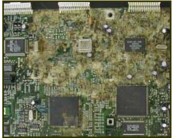
Contamination impacted PC board
