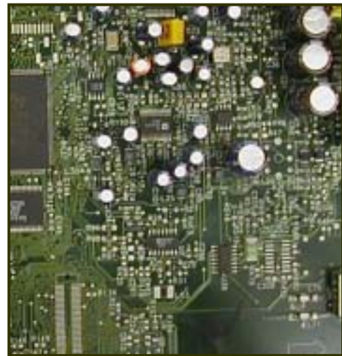
PC board after micro-abrasive blasting
