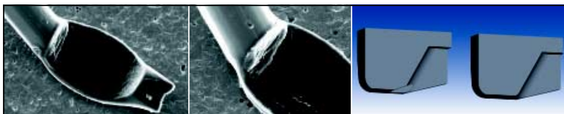
SEM of Bond with Cracked Heel
