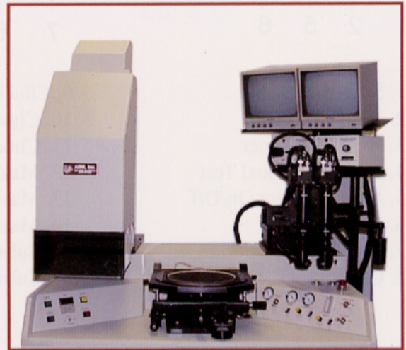
Aligner with Dual CCD Alignment Optics
