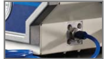
PowderGate® valve – No pinch. More responsive and more consistent abrasive flow
