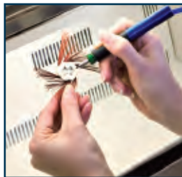
Epoxy removal from probe rings
