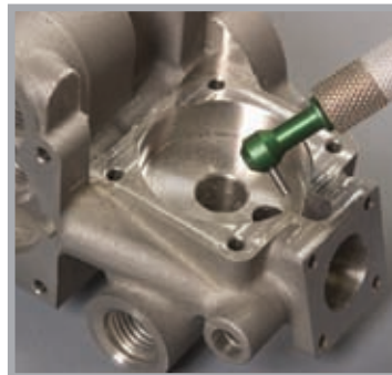
Deburring Ports on Manifolds
