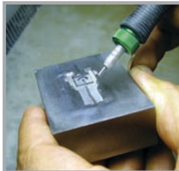
Texturing and Cleaning Mold Cavities
