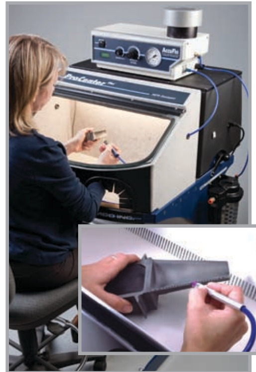
Cleaning Laser Drilled Holes in Turbine Blades
