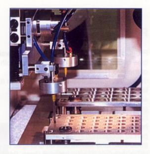
Integrating splitters with a PowerFlo or DirectFlo blaster and the PR1101 Profiler allows multiple nozzle arrays with evenly metered powder flows.
