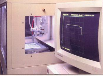
Control of the system is provided by a PC with a Comco bus link to the machine controls and VGA monitor. The menu-driven programming is in a convenient condensed format, with a full screen text editor and the graphics generator, to verify programming or monitor the progress of operating sequences. Programs in inch or metric units are stored for future recall.
