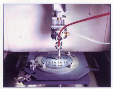
Although the standard nest uses an edge mask to hold flat parts, custom fixturing can be conveniently installed in the abrade chamber.
