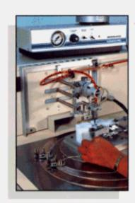
Illustrated at left is a TR4OOO modified to adjust a truck voltage regulator. Once the operator has loaded the nest, the system conducts 3 pre-trim tests, adjusts the voltage to 14V and then conducts 3 post trim tests. Because the volume was only 100,000 regulators per year, the abrasive system, at 1/6 the cost of a laser system, was able to give excellent results at the lowest cost per trim.
