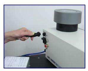
Connecting the MB2300-1 does not require any tools. The footswitch is connected to the back of the timer box and the MB2300-1 plugs into the footswitch receptacle on the back of the blaster.
