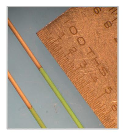
Microblasting consistently provides complete removal of the coating, essential to avoiding the risk of residual contamination.
