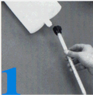
1 Attach static mixer to cartridge.
