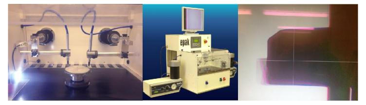
The Epak Electronics Ltd BV6600 Rectifier Beveller is designed to create a profiled edge on a rectifier wafer. The machine uses two Comco Accuflo micro abrasive blasters to process parts from 40mm to 150mm in diameter.
