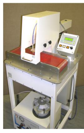
The SA150 Surface Abrader is a system to provide uniform cleaning or abrading of the top surface of parts. Parts are carried on a 150mm wide belt through a closed blast chamber where two micro abrasive nozzles sweep across the top surface of the parts. A Comco Powerflo PF2400 or Directflo DF1400 is integrated into the system to control the abrasive blast functions.
