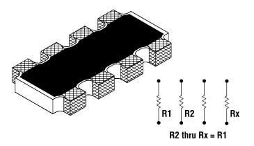
SMR Series of precision resistor networks for fine pitch, surface mount applications. These networks feature a lead pitch of (0.031") and are available in 4 to 16 pin-out styles. The standard value range is 2  $\Omega$  to 10 M $\Omega$ , isolated resistors. Custom configurations are available. Advanced processing techniques, including abrasively trimmed resistors, ensures maximum performance and stability.
