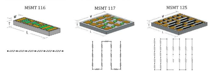
Mini-Systems, Inc. MSMT series chip Multi-Tap resistor arrays provide the design engineer a wide range of resistance values on a single chip. These chips are often used in circuits where **precision adjustments** are required. Connection to associated circuitry is accomplished using wire bonding. The MSMT series offers **high stability, low noise, and low T.C.R.** of Mini-Systems, Inc. proven thin film technology.
