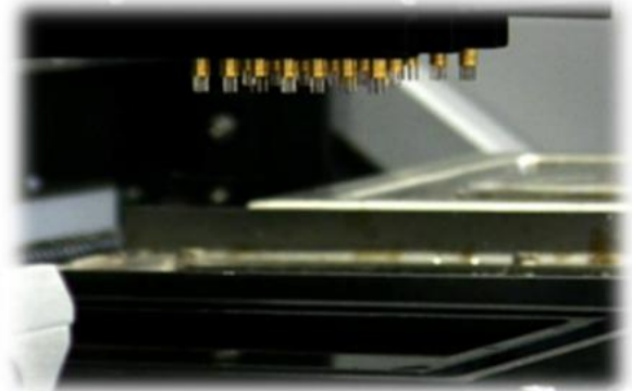
Components in Process | Flux Station
