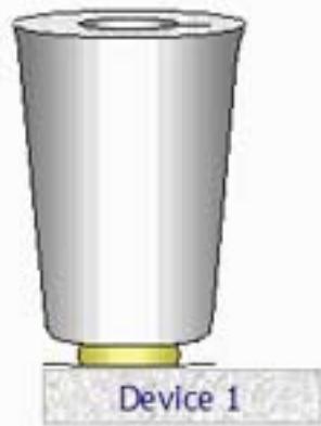
Step 1: Ball bond formation on Device 1
