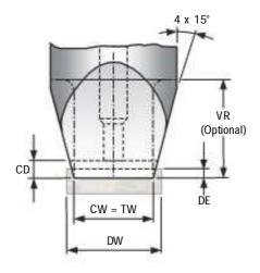
For CH collet, DW is always facing the channel wall and corresponds usually to the longer size
