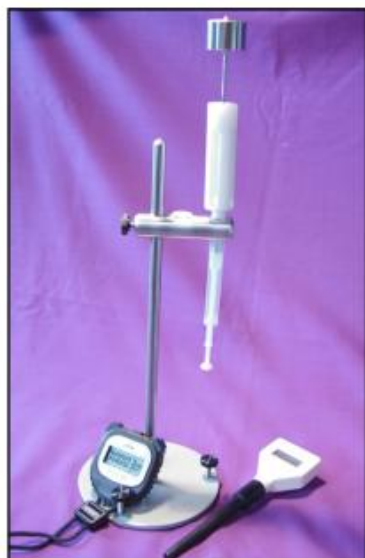
The simple-to-use Portable/Disposable Viscometer (N002-016)
